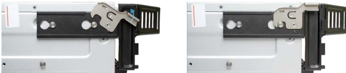
Locate the end of the flex housing with exposed pins. Unclip and open the two tabs closest to the end, allowing the flex housing to compress enough to fit into the bracket holes. Press the flex housing firmly into the bracket until the pins seat in the holes.
