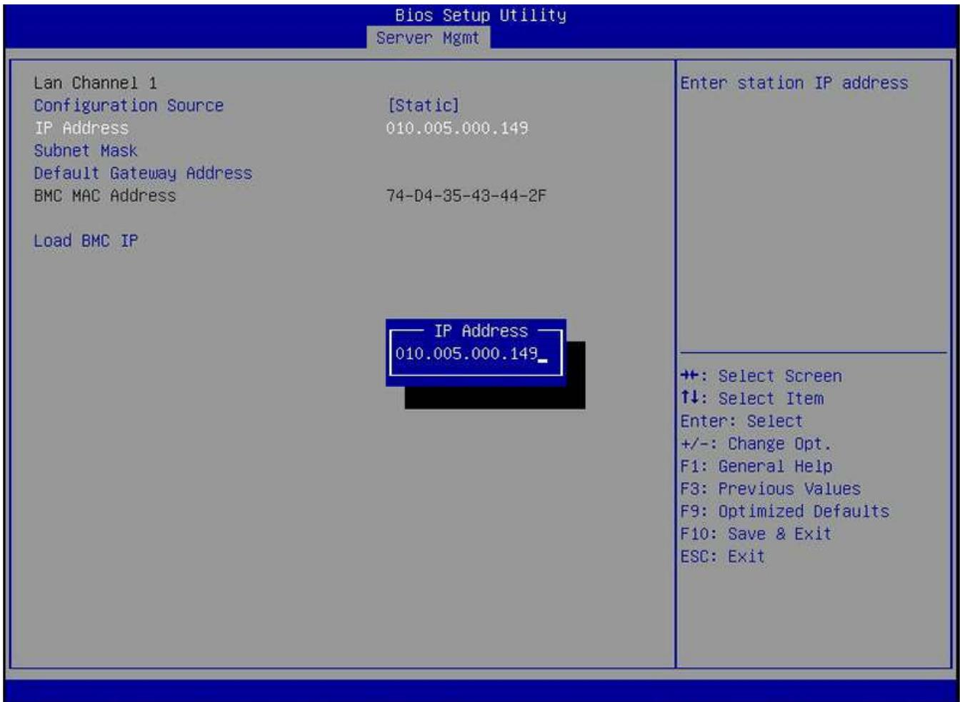
Fig. 2.4: Configuring a Static IP Address
