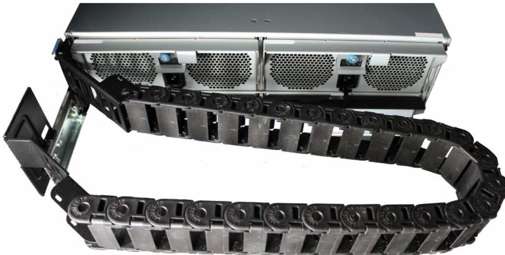
Power and data cables are routed through the flex housing. The tabs can be opened or removed to allow access or space for cable ends. Leave some slack in the cables at both ends to allow for movement of the arm and chassis.
