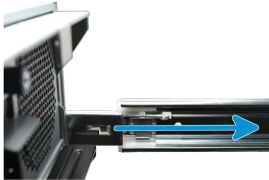
When both cabinet rails are secured inside the rack rails, carefully slide the chassis until the ears are flush with the front of the rack. Tighten both blue screws on the ears of the chassis to secure the unit in the rack.
