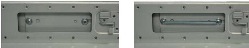
Open the clamp latches on the ends of each rail. Place the rail in the rack with the front end toward the front of the rack, aligning the pins on both ends of the rail with the mounting holes in the rack. Swing the clamp latch closed to hold the rail in place. Use two of the supplied screws to secure the back end of the rail in place. Repeat the process for the second rail.
