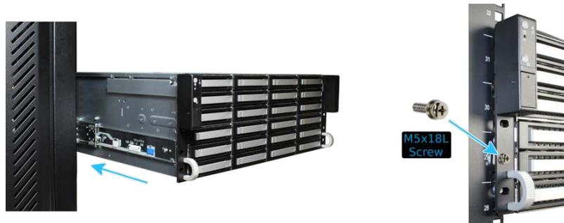
Anchor the unit in the rack on both sides with the M5x18L screws included in the rail kit.
