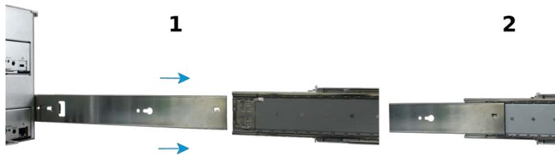
When both cabinet rails are secured in the rack rails, gently push the chassis until it stops halfway in. Slide the blue release tabs on both cabinet rails toward the front of the system while pushing the unit in. Push the chassis into the rack until it is flush with the front of the rack.
