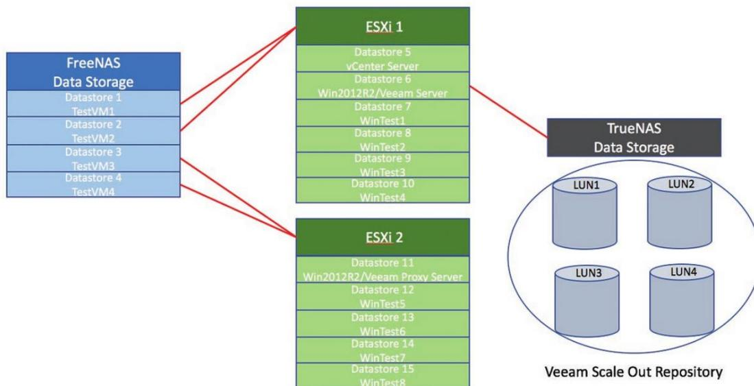
Using a Scale-out Backup Repository, users can link multiple backup repositories (Extents) together to help with performance and load balancing across the various repositories. In the topology above the TrueNAS is broken across four LUNs to act as the scale-out extents. Both the FreeNAS datastore and the TrueNAS backup only used one 10GbE link when connecting to the VMware server pool.
