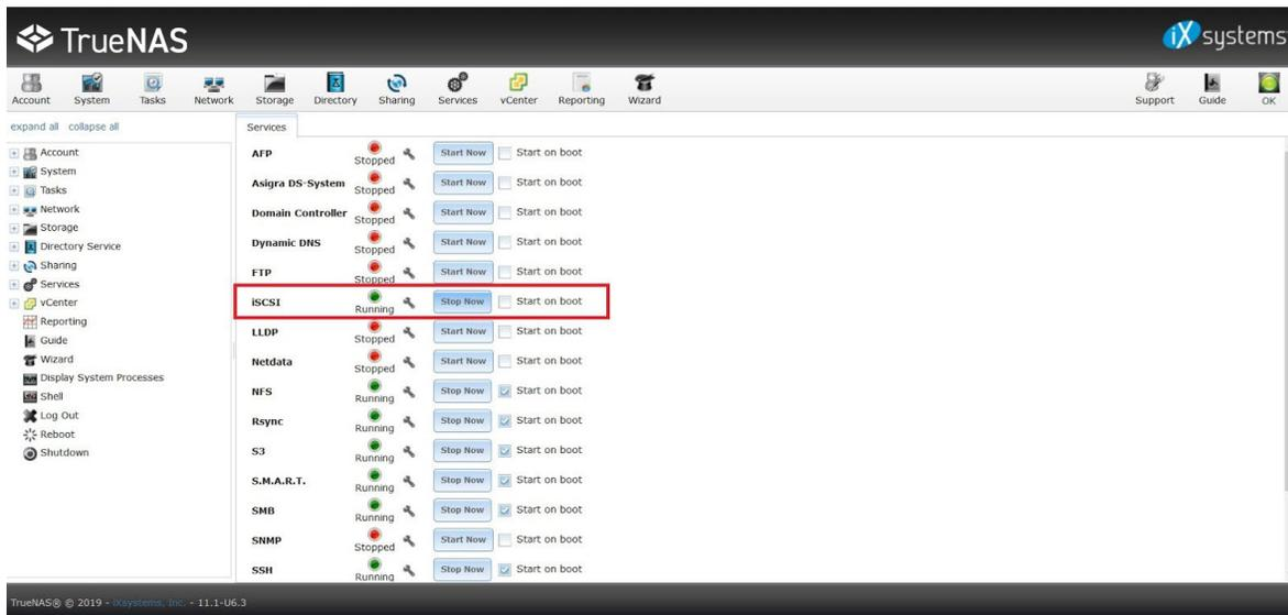
**Step 11:** At this point, the user can mount the iSCSI Target on their Windows Server by starting the **iSCSI Initiator** service in Windows.
