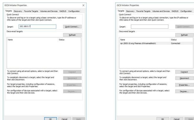
**Step 13:** Once discovered, Windows will see the **Target** as an unformatted, unmapped drive, and users may simply go to the **Administration settings → Computer Management → Storage**, format, and assign a drive letter. Afterwhich, the drive will be shown and accessible, ready to be added as a Veeam backup repository.
