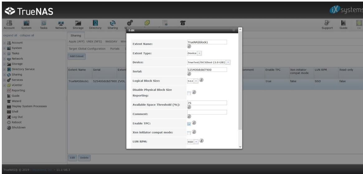
**Step 8:** Creating an **Extent** is where the storage is assigned to this iSCSI share and other options are available. Select the Device type for pairing with a zvol, which is the most supported option. For proper operation as a backup target, it is important **NOT** to enable **Read only** as it will block data writes and your Veeam work will suffer errors.
