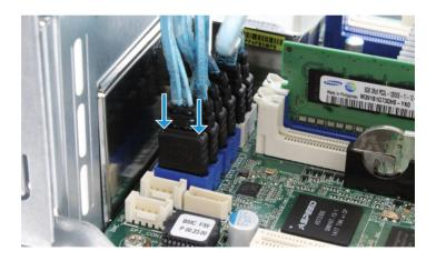
The SATA cables connected to the drive cage might be marked with one to four horizontal lines to show which drive is attached. These marks can be used to sort the cable attachment in drive order.
