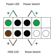
Line up each connector with the correct pins on the header and gently press down until it is fully seated. Make sure wire colors match the diagram above.
