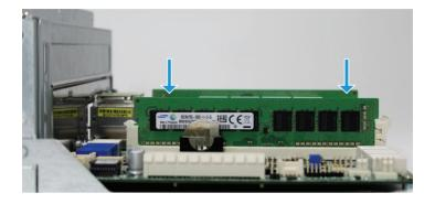
Repeat for the second memory module, which goes in the same color of slot on the other side of the motherboard
