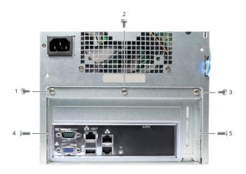
Gently lift and slide the motherboard tray out of the chassis.
