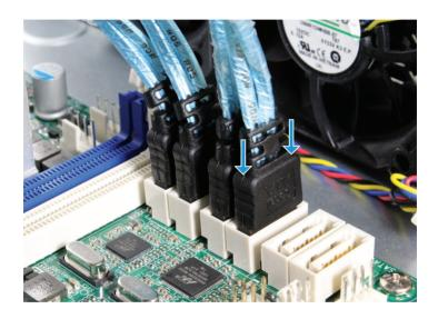
If the optional SSD cache drives are present, connect their SATA cables to the SATAIII\_M2 and SATAIII\_M3 motherboard connectors. It does not matter which cable goes to which connector.
