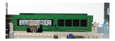
Gently lift the memory module out of the memory slot. If a second memory module is present, remove it also.
