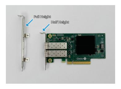
To change the bracket, remove the two retaining screws, exchange brackets, then replace the screws.
