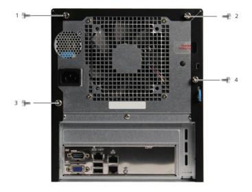
Slide the black metal cover off the back of the chassis.
