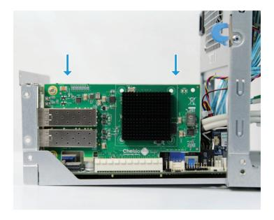
Use the bracket screw removed earlier to attach the network card to the back panel.
