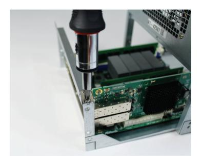
Hold both ends and pull gently upward to remove the NIC from the PCle slot.
