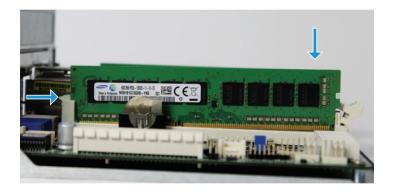
Gently guide the module into the slot, pressing down on both ends of the module until the hinged latch swings in, locking into place.
