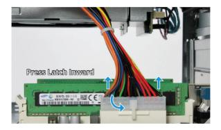
Press in on the upper part of the latch and pull the connector upward to disconnect the power supply cable.
