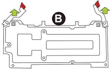
**Pull the handles upwards to remove the CPU Board from the chassis.**
