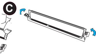
**C.** Press the notches on the ends of the DIMM module inwards to lock it.
