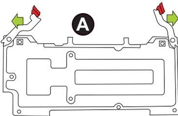
**Press the red latches outwards to unlock the CPU Board**
