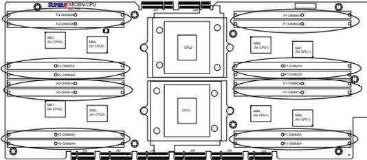
1. Insert the desired number of DIMMs into the memory slots, starting with P1-DIMM #1A. (For best performance, please use the memory modules of the same type and the same speed in the same bank.)
