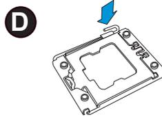
**D.** Once the CPU is fully seated on the socket, press the socket clip down to lock it.
