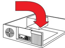
3. Place the baseboard in the chassis, making sure that the mounting holes on the baseboard match the corresponding mounting holes on the chassis.
