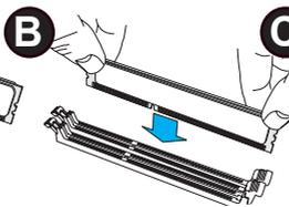
**B.** Insert the DIMM module straight down to the DIMM socket by pressing both ends of the DIMM module at the same time.
