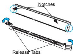
Press both notches straight down into the memory slot at the same time.
