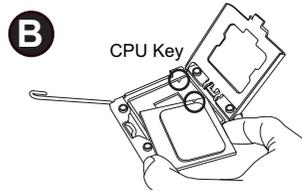
**B.** Align the CPU key with the socket key.
