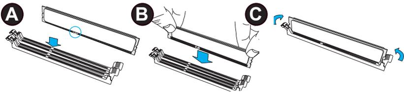
**A.** Align the key on the DIMM module against the key of the DIMM socket.
