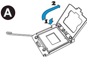
**A.** Press the socket clip down to unlock it. Gently lift the socket clip to open the load plate.
