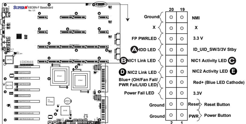
**Overheat (OH)/Fan Fail/PWR Fail/UID LED**
