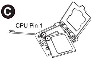
**C.** Align CPU Pin 1 against Socket Pin 1. Once they are aligned, lower the CPU down to the socket.
